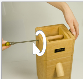
Figure 7 Screw the brake screw back in, adjust the play of the adjusting wheel.
